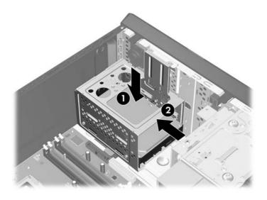
Attach the two screws that secure the hard disk drive cage to the chassis.
